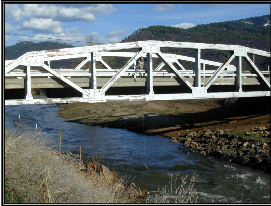
Recording flow using a bridge crane from Deadfall Bridge on Lights Creek, Indian Valley
