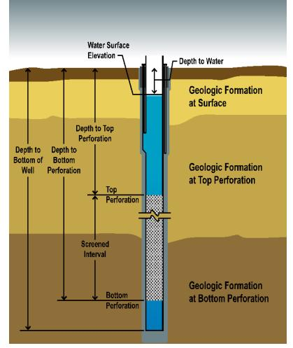
Figure 3-3. Well Completion Diagram
