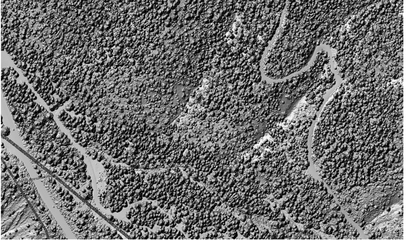
LiDAR Imagery showing forest density and age classes in same area as bare-earth image, above.
