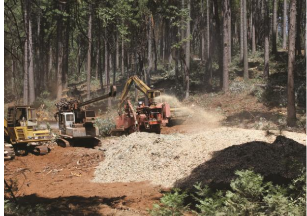
A wood chipper processes woody biomass from a restoration thinning project, Mt. Hope Stewardship Project Plumas National Forest.
