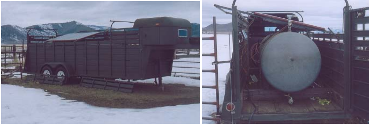
Goodwin Ranch – Solar powered, mobile watering station, for use in Sierra Valley and Red Clover Valley
