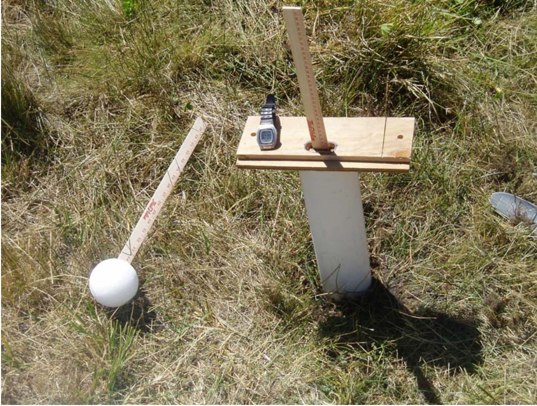
Figure 4. Infiltration field test set-up. White ball is styrofoam and when placed in the 4 inch PVC (protruding from the ground) slowly sinks as water infiltrates the soil. Simple yardstick and stop watch allows for measuring infiltration distance over time.
