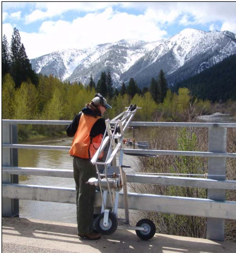
High flow measurements with bridge crane at Taylorsville, April 2010.
