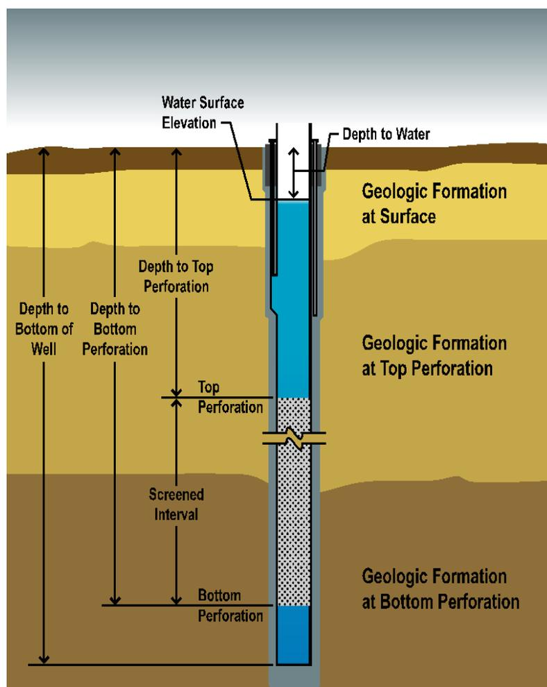
Figure 3-3. Well Completion Diagram
