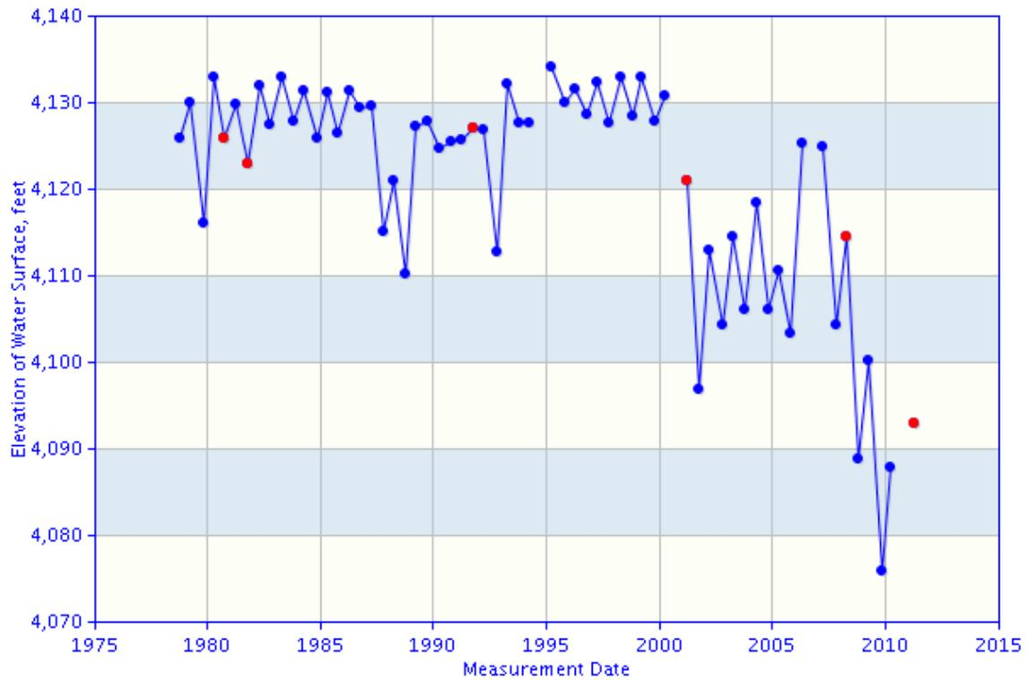
Red data points 2000-2010 – Codes 6,8,9: other, oil or foreign substance in casing, temporarily inaccessible
